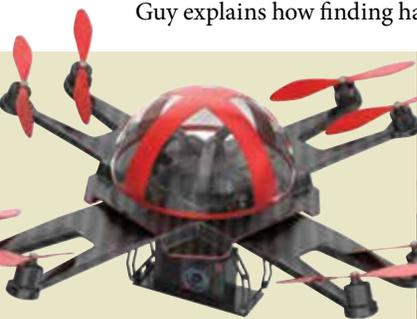
▲ **Hexacopter** This drone uses a thermal imaging camera to find nests.
